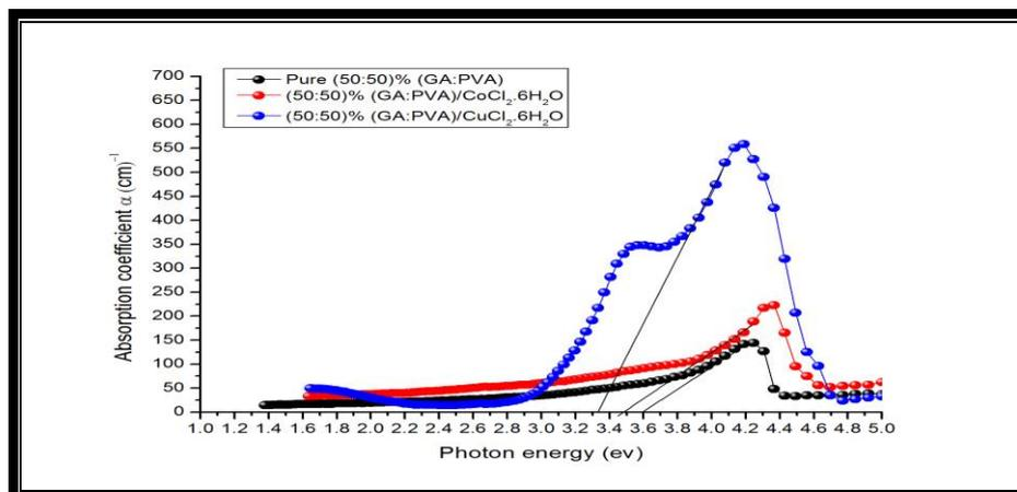
Figure 3. Relation between absorbance coefficient ( $\alpha$ ) versus ( $h\nu$ ) of (50:50)%GA/PVA doping By  $(\text{CoCl}_2 \cdot 6\text{H}_2\text{O})$  &  $(\text{CuCl}_2 \cdot 6\text{H}_2\text{O})$  composite polymer
