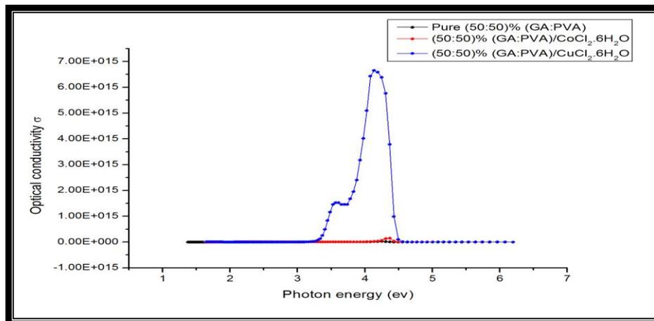
**Figure 7. Optical conductivity of (50:50)%GA/PVA doping By (CoCl<sub>2</sub>.6H<sub>2</sub>O) & (CuCl<sub>2</sub>.6H<sub>2</sub>O).**
