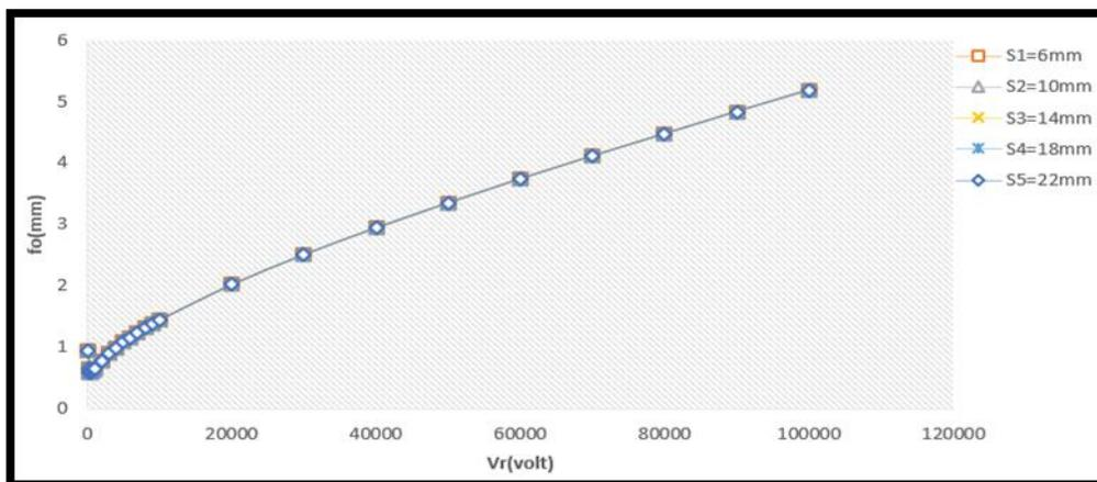
Fig. 6: Focal length as a function of relative corrected acceleration voltage  $V_r$  at a current density of ( $\sigma = 6 \text{ A/mm}^2$ ).
