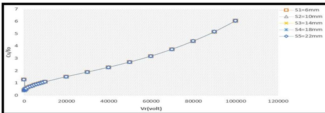
**Fig. 5: Spherical aberration relative to focal length as a function of relative corrected acceleration voltage  $V_r$  at a current density of ( $\sigma = 6 \text{ A/mm}^2$ ).**
