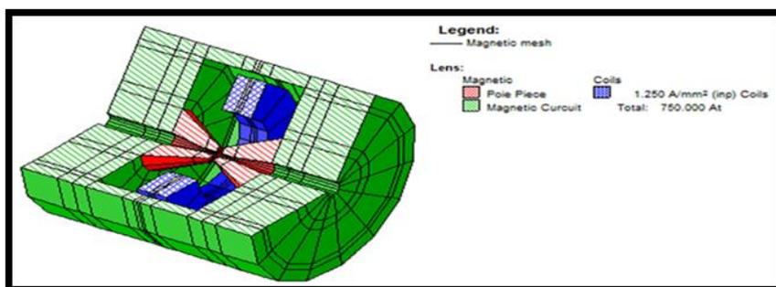
Fig. 2: 3-D magnetic bipolar prototype lens.
