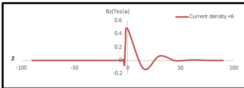
**Fig. 3: Distribution of axial magnetic Flux ( $B_z$ ) as a function of designed lens at current density of ( $\sigma = 6 \text{ A/mm}^2$ ).**
