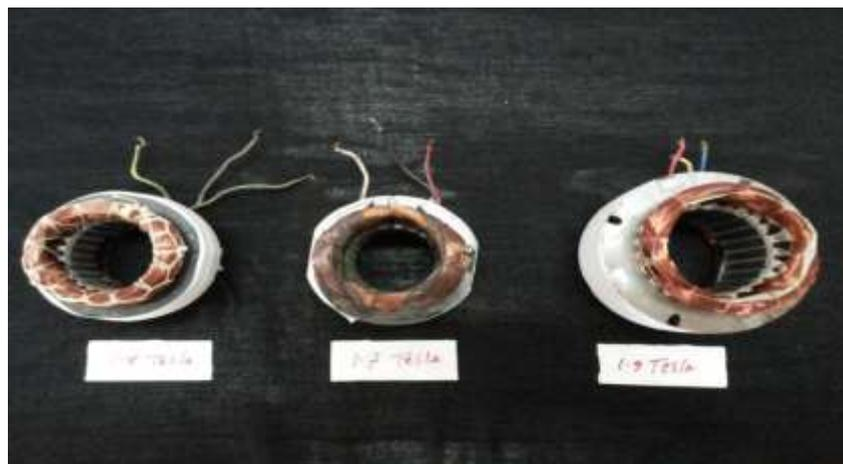
Figure (2) Different electromagnetic field coils
