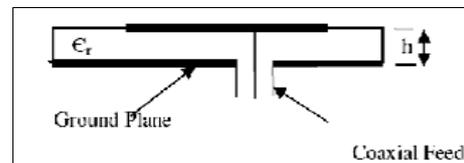
Figure 1. Coaxial feeding method.
