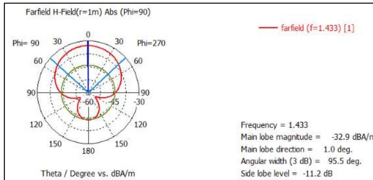
(b) H-plane radiation design for  $f_{\text{res}} =1.433 \text{ GHz}$ .
