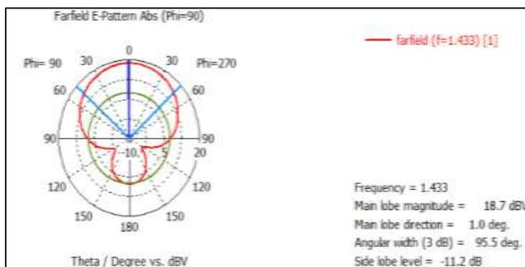
Figure 7.(a) E-plane radiation design for  $f_{\text{res}}=1.433\text{GHz}$
