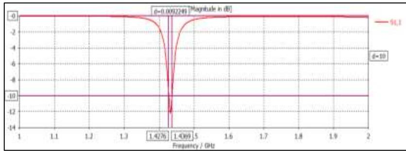
Figure 4. Sham replication coefficient [S11] of the projected microstrip patch antenna.
