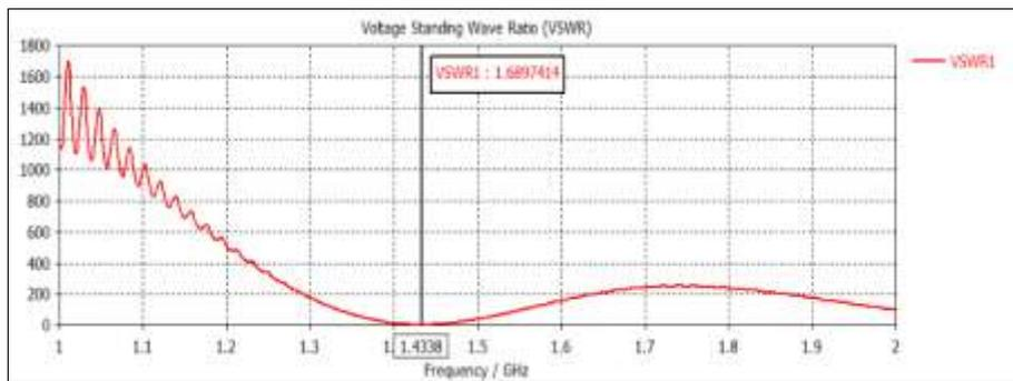
Figure 8. VSWR design for the projected microstrip patch antenna
