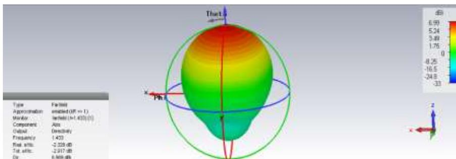
Figure 6. 3D Radiation design for  $f_{rr} = 1.433$  GHz
