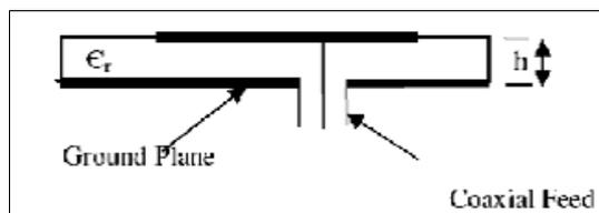
Figure 3. Bottom sight of the projected microstrip patch antenna
